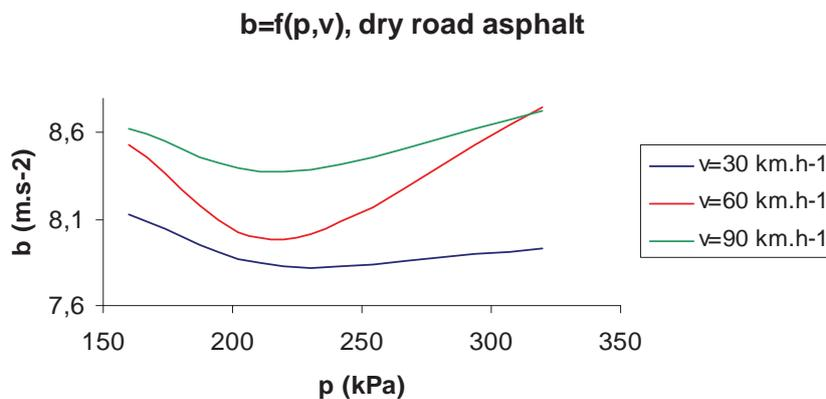
Fig. 7. Maximum braking deceleration dependence on tire pressure and velocity  $v_1$  on dry surface
