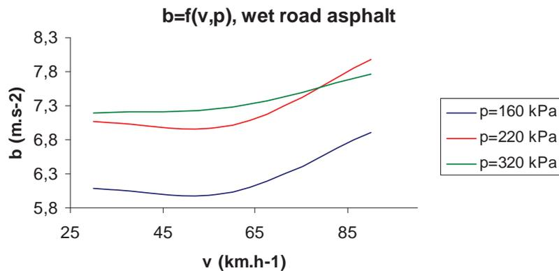
Fig. 10. Maximum braking deceleration dependency on velocity  $v_1$  and tire pressure on wet surface
