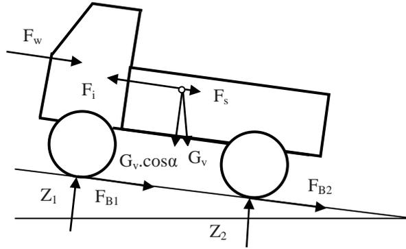
Fig. 1. Vehicle influencing forces at braking
