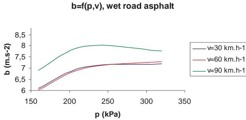
Fig. 8. Maximum braking deceleration dependency on tire pressure and velocity  $v_1$  on wet surface
