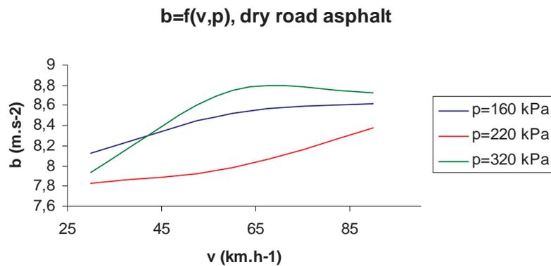
Fig. 9. Maximum braking deceleration dependency on velocity  $v_1$  and tire pressure on dry surface
