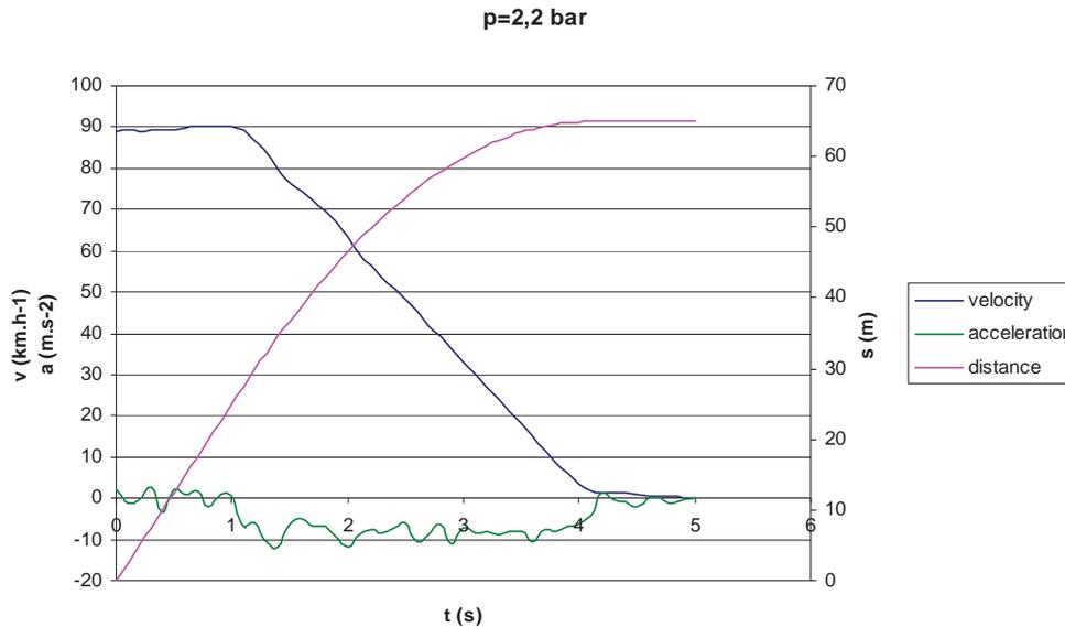
Fig. 6. Measurement from the initial velocity  $v=90 \text{ km.h}^{-1}$
