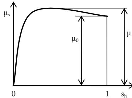
Fig. 2. Slip curve of the wheel
